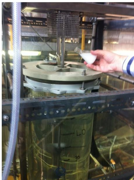
(b) The seeds are poured from the flask into the crystallizer.
