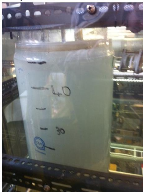
(d) During the cooling down, the solid content in the crystallizer increases and the slurry gets more and more turbid.
