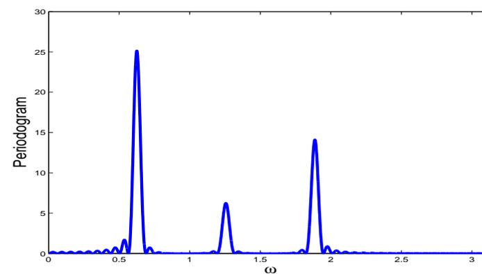
It can be proven that the value at  $\omega_1 = 0.63$ ,  $\omega_2 = 1.26$  and  $\omega_3 = 1.89$  are given by  $\frac{NA_i^2}{4}$  where  $A_i$  ( $i = 1, 2, 3$ ) is the amplitude of the sinusoid of frequency  $\omega_i$ .
