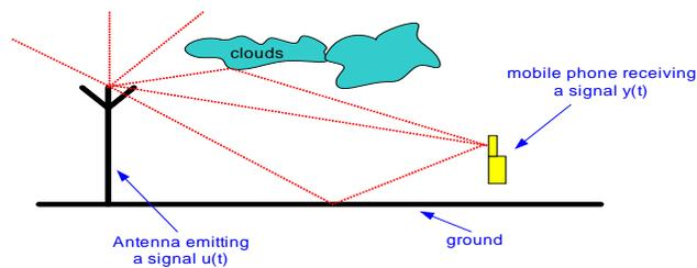
The received signal  $y(t)$  is made up of several delayed versions of the emitted signal  $u(t)$  + noise
