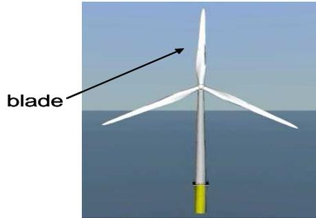
The blades of a wind turbine are subject to high vibration loads due to wind gust, periodic rotations, ...
