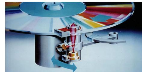
Arm is driven by the current  $i(t)$  of a motor
