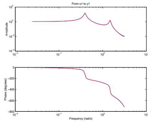
Since the signal  $u$  is p.e. of order  $\geq 6$ ,  $\theta^*$  is unique and the identified  $\hat{\theta}_N$  is a consistent estimate of this  $\theta^* = \theta_0$
