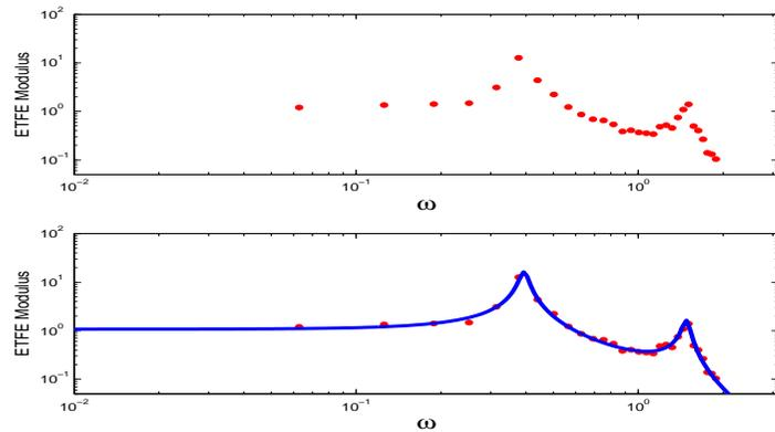
Above plot: the ETFE at the 30 harmonics of  $\omega_0$ ; Bottom plot: the same with the frequency response of  $G_0(e^{j\omega})$  (blue)
