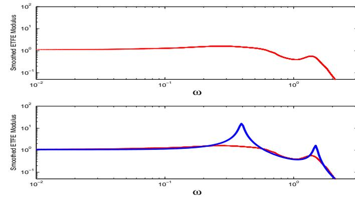
Above plot: the smoothed ETFE at  $\omega_k$ ; Bottom plot: the same with the frequency response of  $G_0(e^{j\omega})$  (blue)
