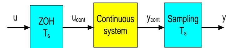
The system is excited via the discrete sequence  $u(t)$   $t = 0, 1, 2, \dots$  generated by a PC
