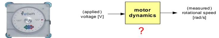
Determine a model of the dynamical relation existing between the voltage  $u(t)$  driving the motor and the angular speed  $y(t)$  of the rotor
