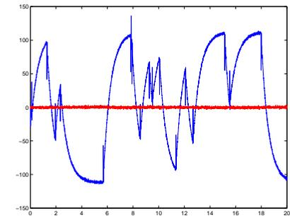
$\epsilon(t)$  contains not only the model inaccuracy, but also the noise acting on the system
