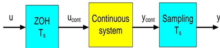
The continuous output  $y_{cont}(t_c)$  ( $t_c \in \mathbb{R}$ ) of the system is sampled with sampled time  $T_s$
