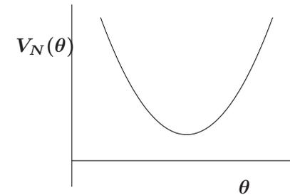
$\hat{\theta}_N = \arg \min_{\theta} \frac{1}{N} \sum_{t=1}^N (y(t) - \phi(t)^T \theta)^2$  can be determined analytically using:
