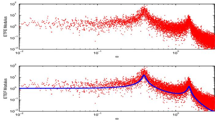
Above plot: the ETFE at  $\omega_k$ ; Bottom plot: the same with the frequency response of  $G_0(e^{j\omega})$  (blue)
