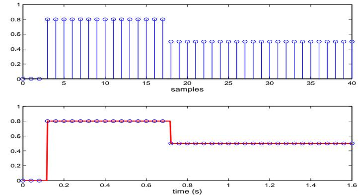
The continuous signal  $u_{cont}$  is then filtered by  $G_0(s)$  delivering the continuous signal  $y_{cont}$  (upper plot, red). This continuous signal is then sampled with a sample period  $T_s = 0.04s$ . (upper plot, blue circle). This delivers the discrete sequence  $y(t)$  of 41 samples ( $t = 0 \dots 40$ ) (bottom plot)
