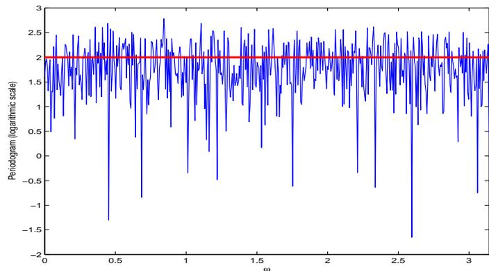
$\hat{\Phi}_u^N(\omega)$  is an erratic function fluctuating around  $\Phi_u(\omega)$
