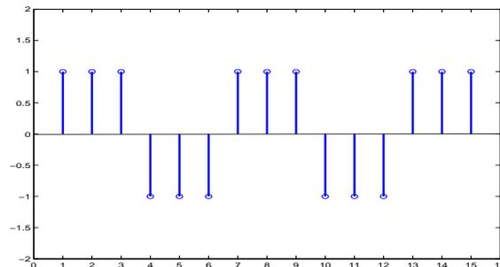
$$\begin{array}{llll} R_u(0) = 1 & R_u(1) = \frac{1}{3} & R_u(2) = -\frac{1}{3} & R_u(3) = -1 \\ R_u(4) = -\frac{1}{3} & R_u(5) = \frac{1}{3} & R_u(6) = 1 & \text{etcetera} \end{array}$$
