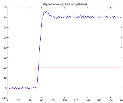
From this behaviour, we can conclude that  $G_0$  has a limited order and from a detailed observation, we see that the delay is  $n_k = 3$
