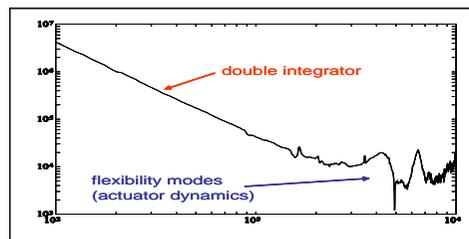
For a bandwidth of  $\approx 1000 \text{ Hz}$ , the mechanical modes can no longer be neglected and should be tackled by the controller
