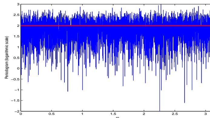
Example 2: we have collected  $N = 100$  time-samples of  $u(t) = \sin(0.63t) + \frac{1}{2}\sin(1.26t) + \frac{3}{4}\sin(1.89t)$  (fundamental period = 10 time-samples):
