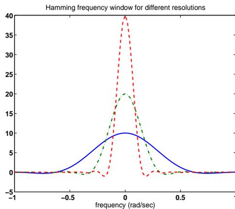
$W_{\gamma}(\omega)$  of Hamming window for  $\gamma = 10$  (solid),  $\gamma = 20$  (dash-dotted) and  $\gamma = 40$  (dashed).
