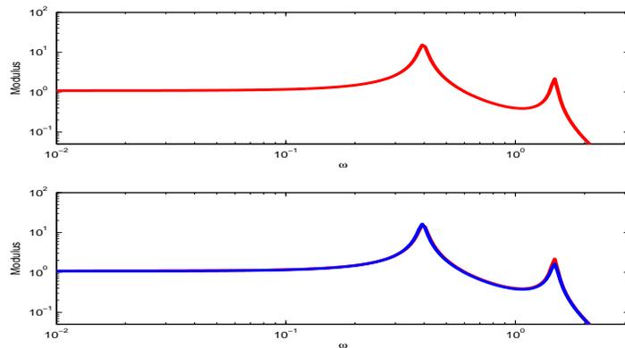
Above plot: frequency response of the identified model; Bottom plot: the same with the frequency response of  $G_0(e^{j\omega})$  (blue)
