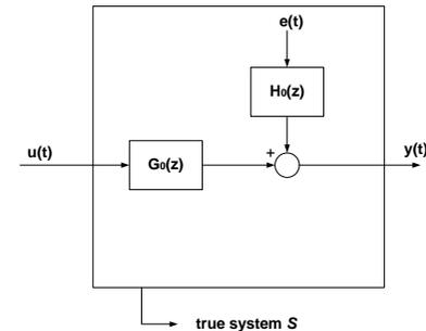
$G_0(z)$  and  $H_0(z)$  are two unknown linear transfer functions in the  $\mathcal{Z}$ -transform ( e.g.  $G_0(z) = \frac{3z^{-1}}{1+0.5z^{-1}}$  and  $H_0(z) = \frac{1}{1+0.5z^{-1}}$  )
