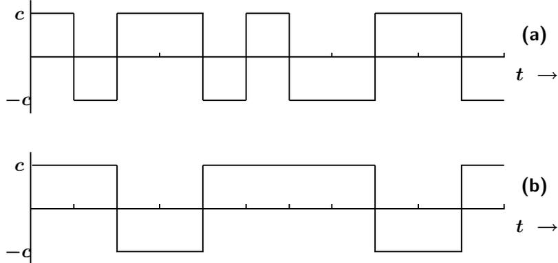
(a) Typical RBS with clock period equal to sampling interval ( $\nu = 1$ );
