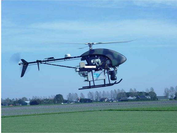
Figure 1.8: NLR's mini-UAV project (2004-2006) based on a modified Bergen Industrial Twin helicopter.
