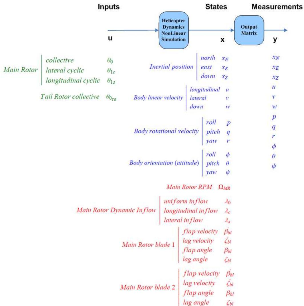
Figure 2.2: Helicopter Inputs  $u$  (in green), States  $x$  (in blue the rigid-body states, in red the main rotor states), and Measurements  $y$  (measured states).
