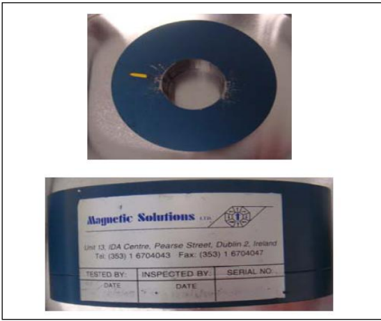
Fig.1. Top and side views of the Halbach cylinder
