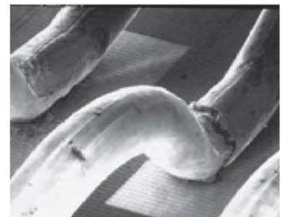
Figure 23: Wire cracking [19]
